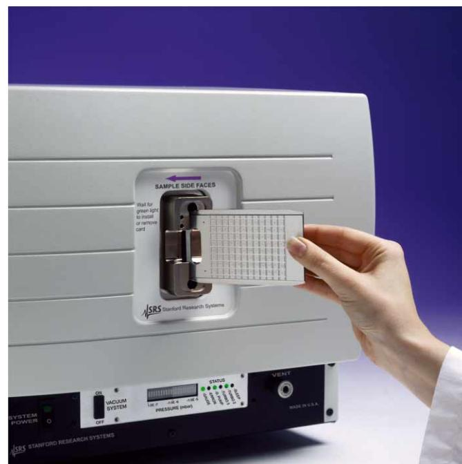
sample card is also available that allows placement of electrophoresis gels directly onto the card. Profiler's software has a sophisticated video imaging algorithm that maps the target area of each sample so laser shots aren't wasted on blank areas of the sample plate. This translates directly into high throughput. Firing 64 laser shots per sample spot, Profiler can acquire data on a card of 96 sample spots in about a half hour.
