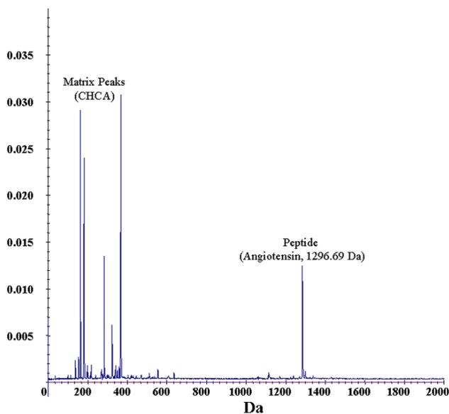
Profiler's discrete dynode detector allows you to display matrix and analyte peaks simultaneously without the need for matrix blanking.
