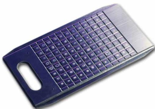
batch of samples, can be analyzed in any particular order and with different protocols (mass range, extraction voltage, etc). Calibration standards can be distributed throughout the sample card and used to dynamically calibrate the mass axis during unattended data collection. A second type of
