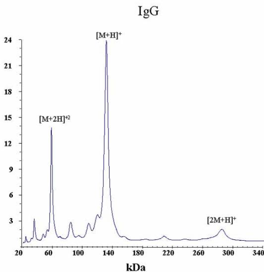
Profiler's high mass range capability is demonstrated by this mass spectrum of 1 pmole of Immunoglobulin G antibody. The dimer ( $2M+H$ )<sup>+</sup> ions is clearly visible at 300 KDa.
